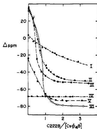
**Figure 2.** Plot of cesium-133 chemical shift vs. C222B/CsBPh<sub>4</sub> mole ratio in different solvents. Concentration of CsBPh<sub>4</sub> is 0.01 M in all cases: (I) DMF, (II) PC, (III) Me<sub>2</sub>CO, (IV) Me<sub>2</sub>SO, (V) MeCN, (VI) PY.
